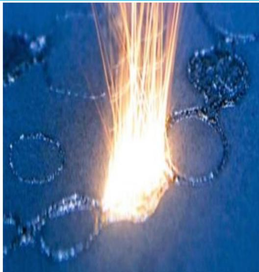
LPS involves a powder (singular or a two part mixture), a scraper to displace the powder . Smaller particles with lower melting points bind the larger particles used for structuring . These SLS/LPS could then be alternated throughout the initial 20m and the full 100m as a way to maintain a constant lining density.
