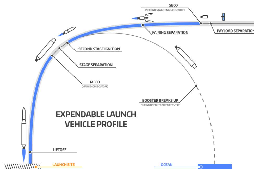
trajectory. Launch profile of Falcon 9 (Gardi & Ross, 2016) sired altitude at which to circularise, the rocket will have to begin its gravity turn at a sufficient altitude. Because
