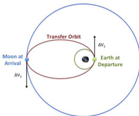
In the process of getting to the Moon, the engines perform a prograde (accelerating in the direction of travel) at a given point in the LEO (MoonConnection, 2016), to bring the apoapse, which is furthest point in orbit from Earth (Bruce, 2009), approximately 3 days ahead of the Moon's orbit. The velocity must be scaled up to over  $11.2 \text{ kms}^{-1}$  order to bring the apoapse up sufficiently. Simply put, this requires an additional
