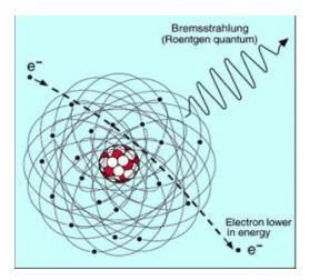
The issue with gamma radiation being shielded by high density materials is that high level beta radiation is shielded by low density materials. This is due to a radioactive process known as bremsstrahlung. As shown in figure 2<sup>10</sup>, this is where a high speed particle (electron) passes through a magnetic field or interacts with another charged particle and decelerates very quickly. When this happens, electromagnetic radiation is
