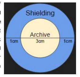
would give a 30mm diameter to the archive itself. The DNA samples, which are likely to be much smaller than the digital archive, should also have their own shielding built into their capsules.
